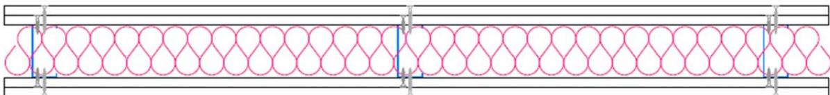
This assembly produces a result in the lab of STC-58. This is in a laboratory setting with floor and ceiling flanking paths reduced to their minimum. It is not realistic to assume that you will obtain this degree of isolation in the field.
