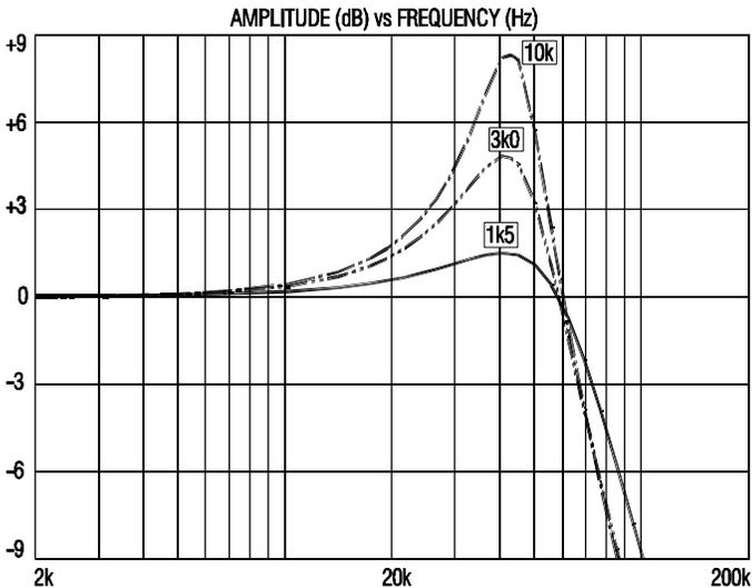
Figure 3 - **Damping Effect of Preamp Input Impedance**
