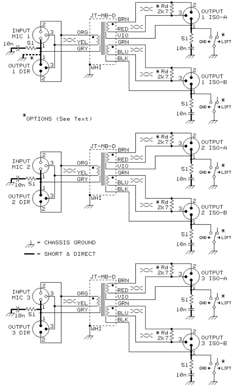
Figure 7 - Complete 3-Channel, 3-Way Splitter
