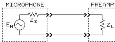
$$\text{INPUT VOLTAGE AT PREAMP } E_p = E_M \times \frac{Z_L}{Z_S + Z_L}$$
