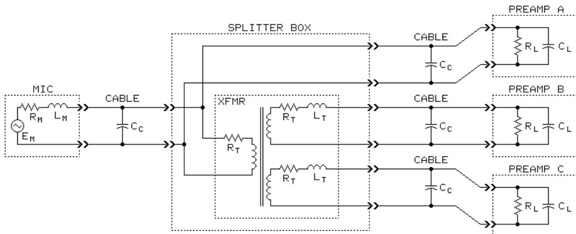
Figure 2 - Simplified Schematic for Estimating Losses and Bandwidth
