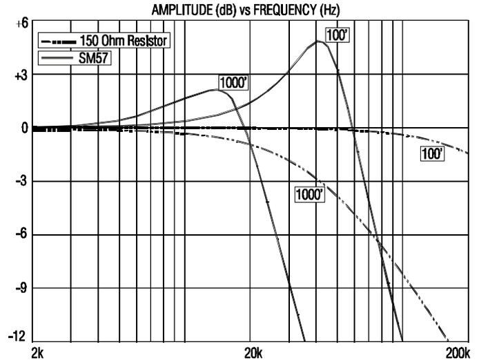
Figure 4 - **Effect of Cable Length on Response**
